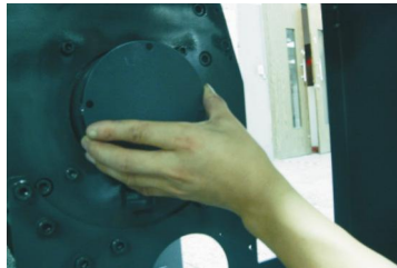
Picture 3-7: Installation of Bearing Cover Plate
