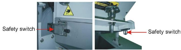
Picture 2-3: Safety Switch
