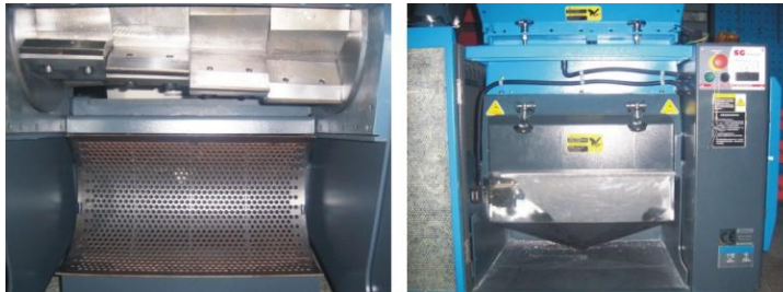
Picture 3-9: Installation of Screen, Screen Bracket and Storage box
