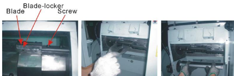
Picture 6-1: Disassemble the rotary blades
