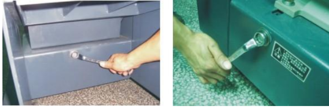
Picture 6-3: Adjustment of V-belt
